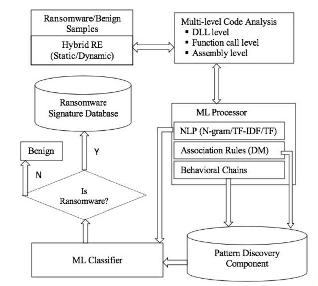
Fig: The overall backend architecture for AI-powered ransomware detection framework
