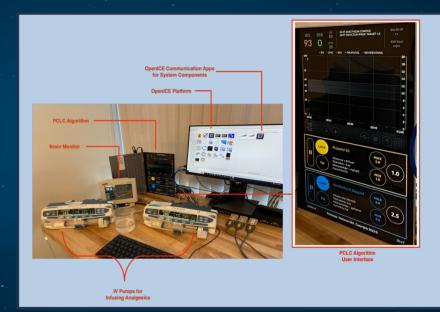
OpenICE-based hardware-in-the-loop testbed for a PCLC anesthesia system
