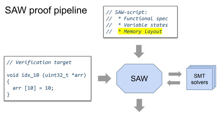
Result: verified / failed (memory safe, functionally correct, ...)
