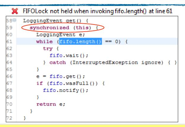
The programmer determines that the code is wrong and fixes line 59
