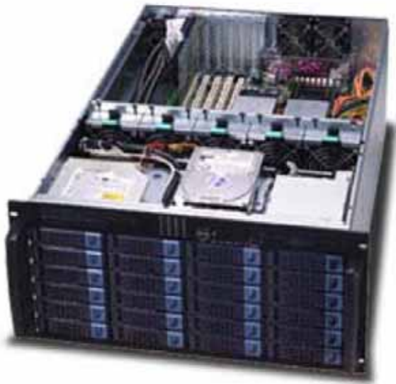
Figure 3-8: A storage element of the Pan-STARRS data pipeline. The storage uses only commodity components [25].
