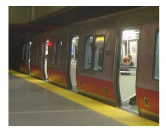
System Hazards H-1: Doors close on a person in the doorway H-2: Doors open when the train is moving or not at platform H-3: Passengers/staff are unable to exit during an emergency
