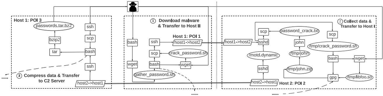
**Figure 4: Critical components generated by DEIMPACT for the “Shellshock” attack (non-critical edges are omitted). DEIMPACT generates critical components for the three POI events and takes the union of the generated critical components, which covers all the attack steps as described in Section 5.1.2.**
