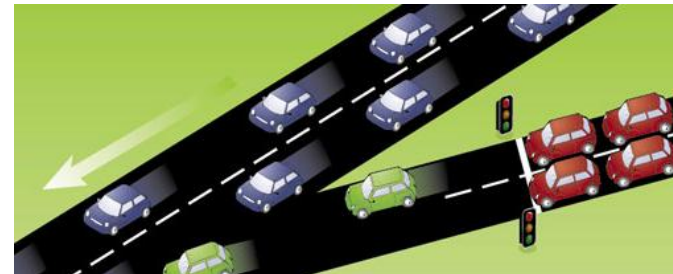
Figure 8: Ramp metering diagram (From New Zealand Transit Agency)
