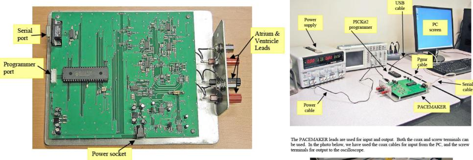
You should try and identify components on the board. The Atrium and Ventricle leads can be connected by coax or by simple wires with a common ground. We suggest using simple wires.
