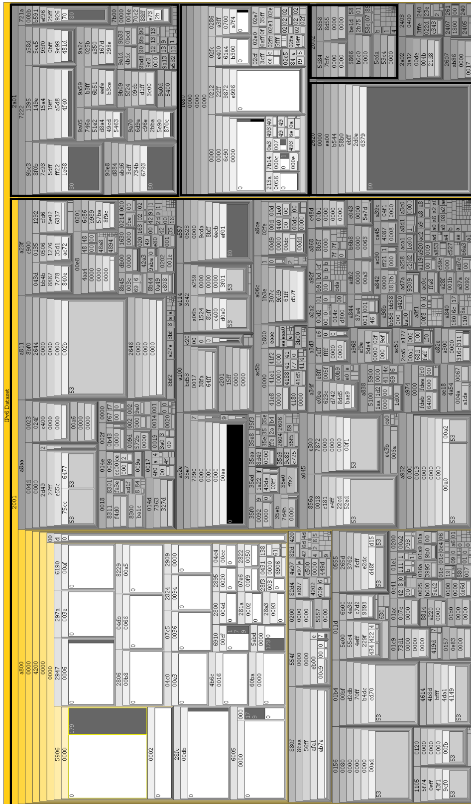
Figure 6.3: A treemap representing IPv6 source address, destination port and packet count. Colour key: ICMP (white), TCP (dark grey), UDP (light grey), other protocols (black). Best viewed in colour.
