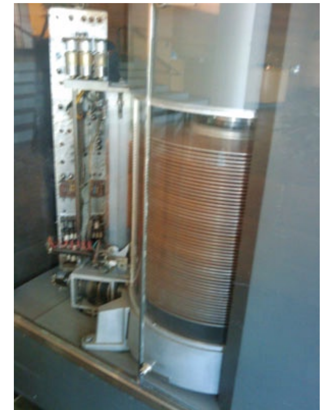
One of the first commercial disk drives from IBM. It has a 5 MB capacity and it's stored in a cabinet roughly the size of a luxury refrigerator. In contrast, a 32 GB microSD card measures around 5/8 x 3/8 inch and weighs about 0.5 gram.
