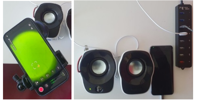
Figure 13. Experimental setup. The video camera of an iPhone 13 Pro Max is directed (through a lens) at the power LED of Logitech Z120 speakers that are connected to a USB hub used to charge a Samsung Galaxy S8 (which contains the SIKE key).
