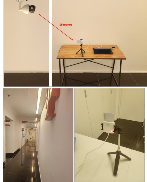
Figure 8. Experimental setup. Top: The video camera located 16 meters away from the smartcard reader. Bottom: As seen on the left, the smart card reader (pointed at by the red arrow) is pictured from 16 meters away. On the right is an image of the smart card reader’s power LED.
