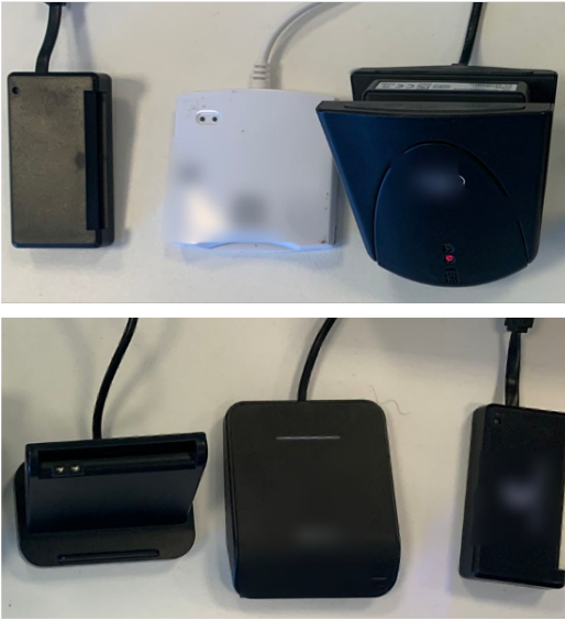
Figure 7. An obfuscated picture (we blurred the visual identifiers of the manufacturers) of the six smartcard readers, from which we recovered ECDSA keys by analyzing their power LED.
