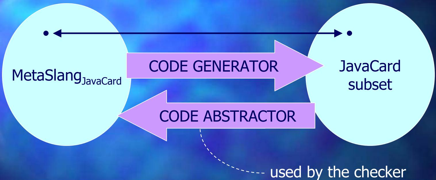
code generator checks that spec is in MetaSlang<sub>JavaCard</sub> and maps it to corresponding Java Card program
