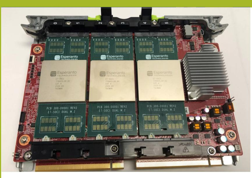
1000, RISC-V\* processors on a single 7nm chip.
