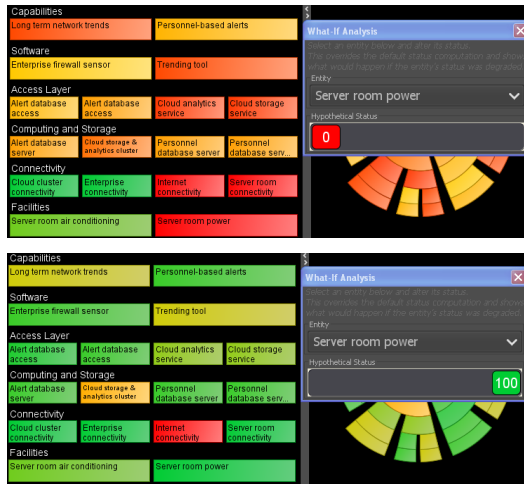
Figure 9. “What-if” analysis provides a predictive analysis capability. The two figures show the predicted status of the system when “server room power” is unavailable and when it has full power.
