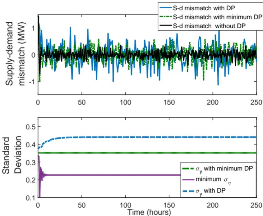
Distributed Frequency Control in the Smart Grid with a DP mechanism.
